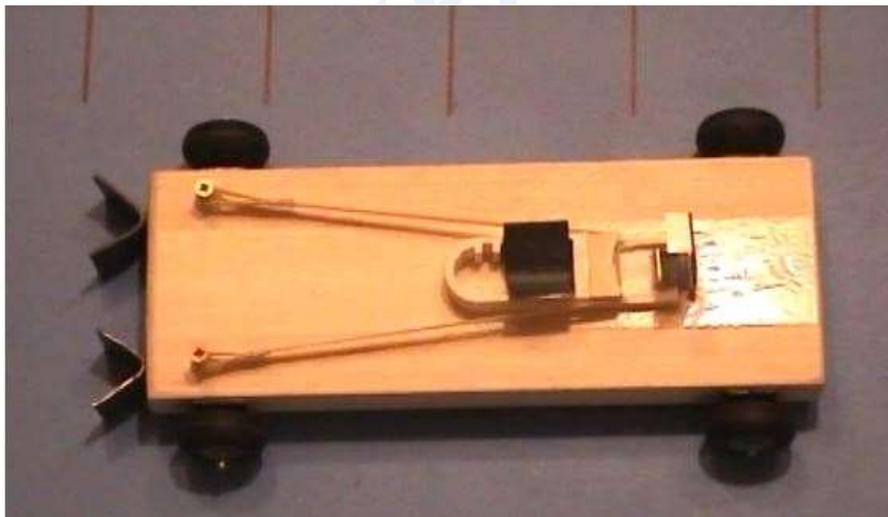
The carriage was placed at the bottom of a sloping board (approximately 5% slope) and the distance travelled observed when 'firing off' 40, 80 & 120gm lead weights.
