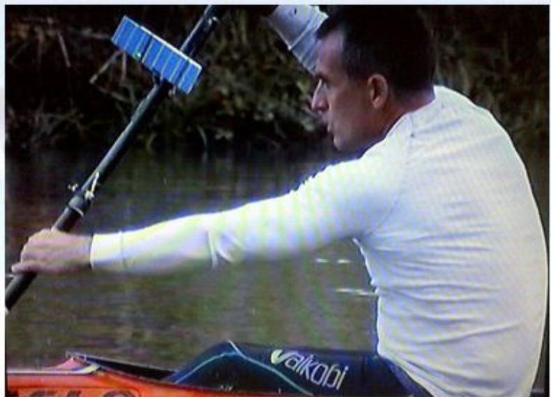
**'Force Meter'** - A stiff carbon rod is clamped just 'inside' of one of the paddler's hand positions. The far end of the rod does not move with the paddle shaft as it bends under load. This difference in displacement is used to move a small mirror, reflecting a laser beam on to a 'scale' at the clamped end of the stiff tube.
