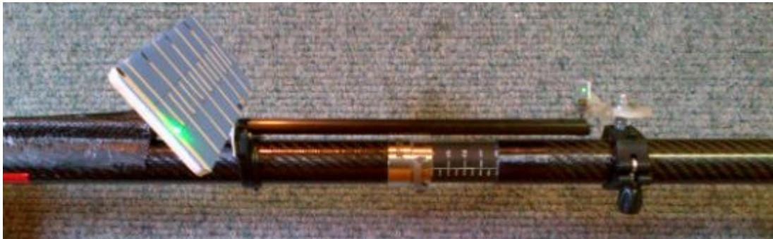
After the paddling / video session, the paddle is incrementally loaded with weights at the 'lower hand' position while being supported at the upper hand position and an area close to the assumed blade centre of pressure. A 'translation table' can then be created to convert the 'videoed' scale readings to Kgf.
